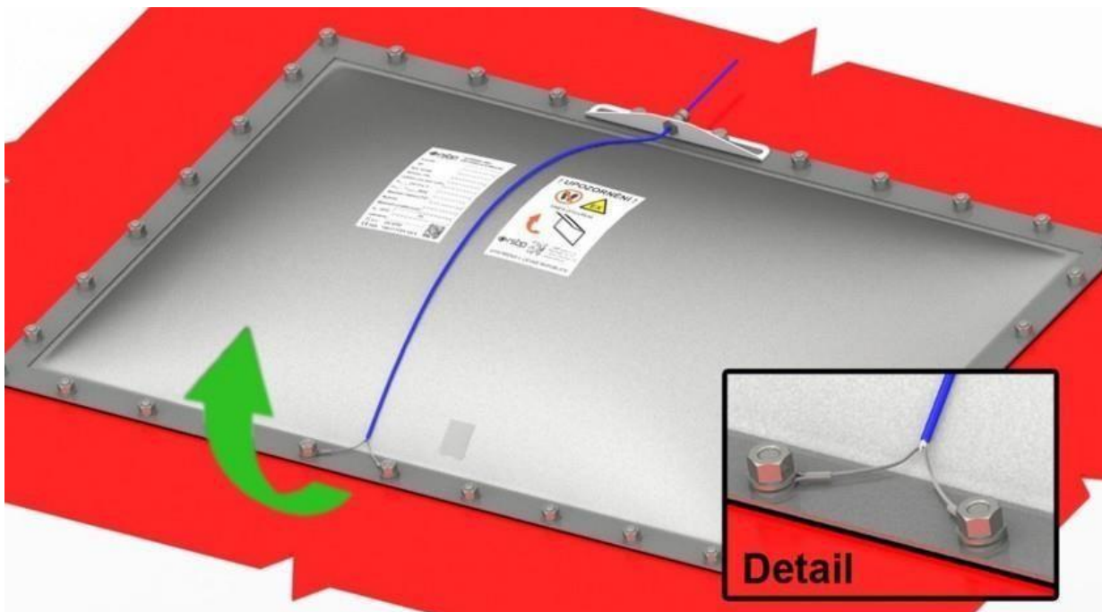
Fig. 24 - Correct position of the G3 opening indicator in relation to the opening side of the Vent PRO S
